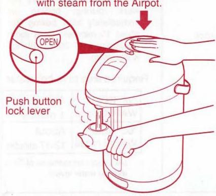
Set the push button lock lever to the "OPEN" position and press the push button to pour boiled water.
